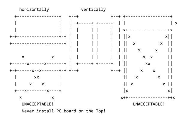
The drive may be mounted horizontally with the PC board down or on either side. Mounting vertically on either end is a prohibited orientation.
